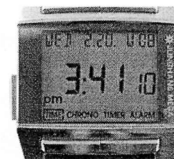
FIGURE 1.8. Junghans Mega 1000 Digital Radio Controlled Watch. There is no good conceptual model for understanding the operation of my watch. It has five buttons with no hints as to what each one does. And yes, the buttons do different things in their different modes. But it is a very nice-looking watch, and always has the exact time because it checks official radio time stations. (The top row of the display is the date: Wednesday, February 20, the eighth week of the year.) (Photograph by the author.)
